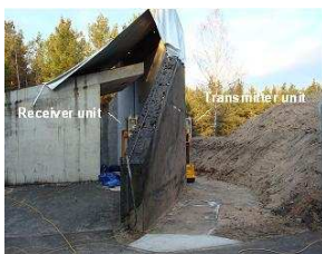
Figure 1. Determination of the electromagnetic properties of a 50 cm thick steel reinforced wall segment with UWB technique
