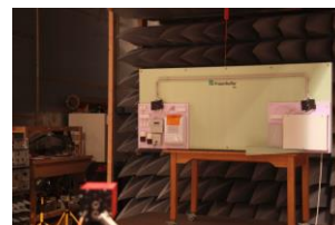
Figure 1. Test setup fixed on rigid foam with groups and cable harness.
