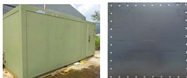
Figure 1. Shielding room and PoE(Point of Entry)
