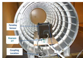
Figure 4. Low level measurement on an internal structure.
